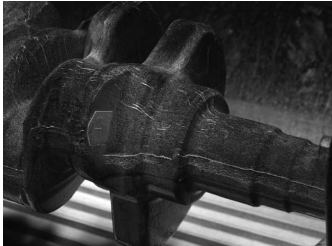
FIG. A1.4 Crankshaft with Various Longitudinal Indications
