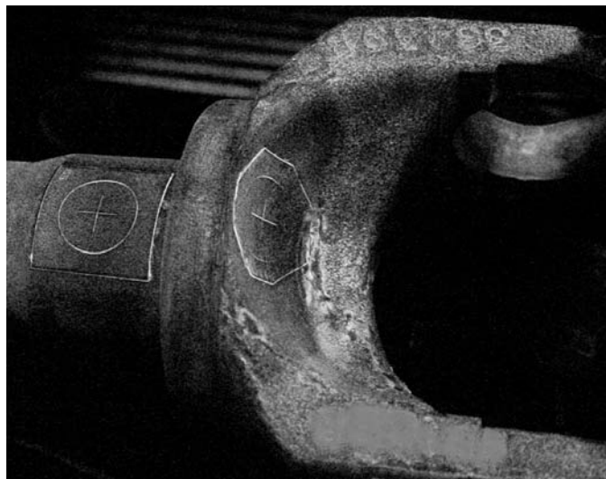
FIG. A1.6 Yoke Showing Balanced QQIs
