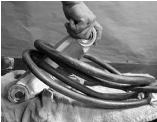
FIG. 9 Cable Wrap Magnetization
