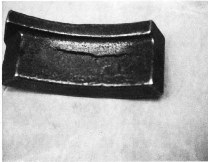
FIG. A1.17 Indications of a Near-Surface Discontinuity (Produced by Prod Magnetization, HWDC Continuous)
