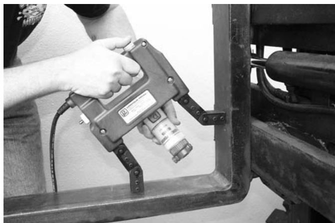
FIG. 1 Yoke Method of Part Magnetization
